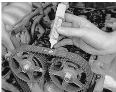
Fig. 21: Mark the direction of rotation on the timing belt in case you need to re-install the original belt
