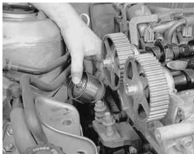
Fig. 29: If necessary, or in case of high mileage, remove the tensioner pulley by removing the lockbolt
