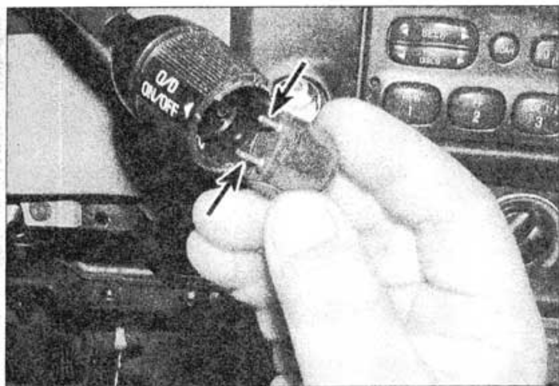
9.3b The transmission control switch simply pulls out of the shift lever - check the pins for continuity when the button is depressed
