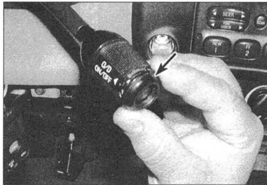
9.3a Pry the cover (arrow) off the end of the shift lever top expose the transmission control switch
