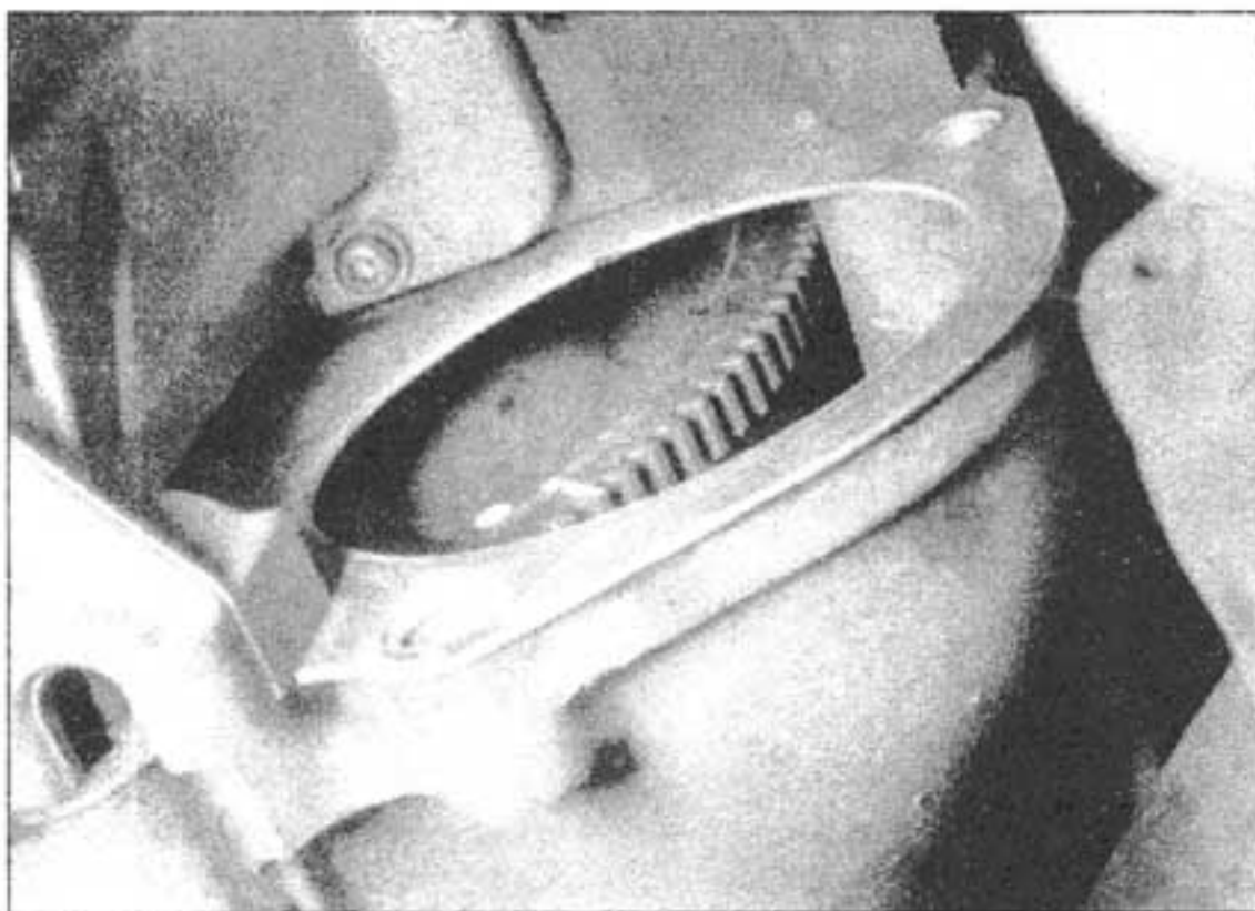
12.6 Mark one of the torque converter studs with white paint and make a corresponding mark on the driveplate so the torque converter and driveplate can be reassembled in the same relative positions
