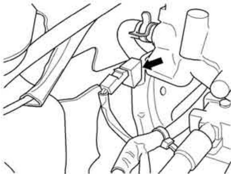
Fig. 26 COIL CAPACITOR - 2.4L TURBO
