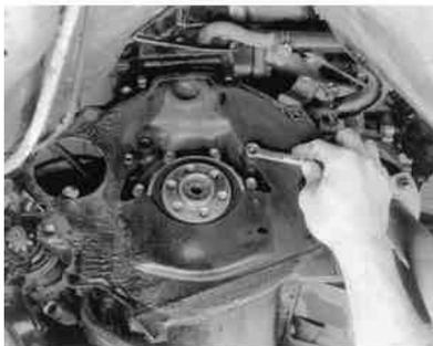
Fig. 2: Loosening the rear main seal attaching bolts
